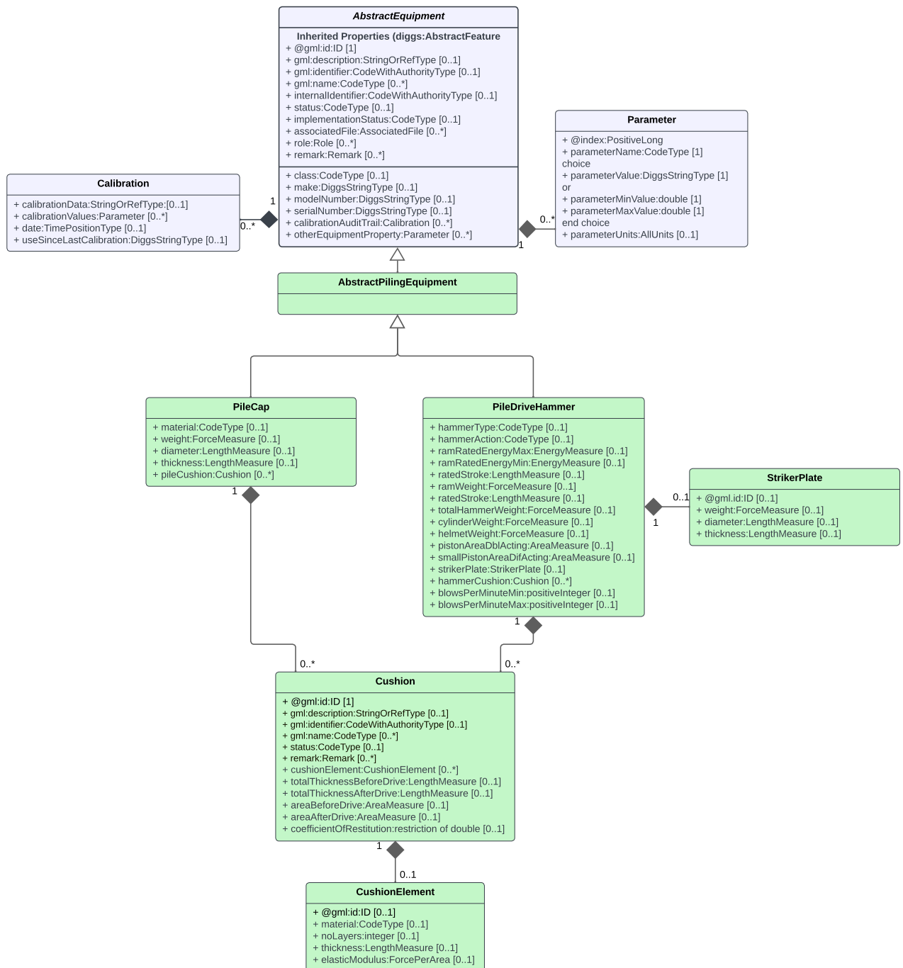
Figure 3. UML diagram illustrating proposed equipment objects use when storing and transferring data from pile driving activities (green). Light-blue colored objects have been previously developed. The newly proposed PileDriveHammer and PileCap objects inherit properties from their parent AbstractEquipment object.
