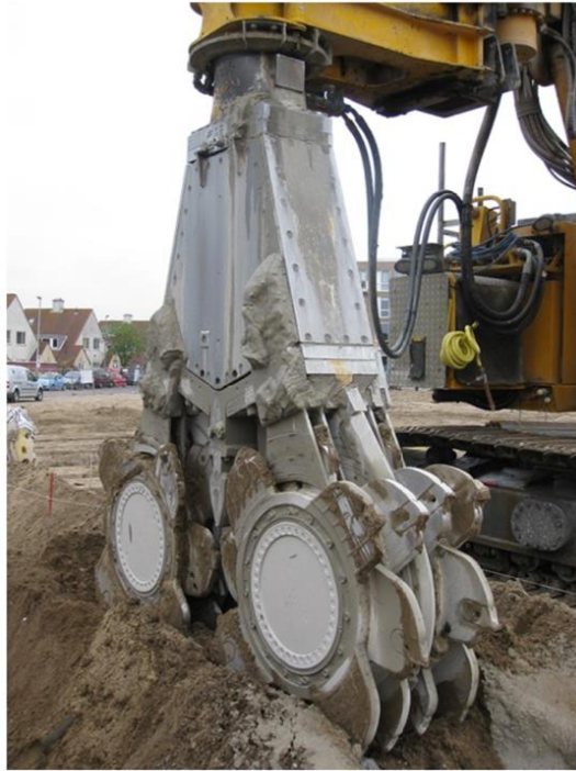
Figure 3: Image of the cutter soil mixing tool (Bellato et. al., 2017).
